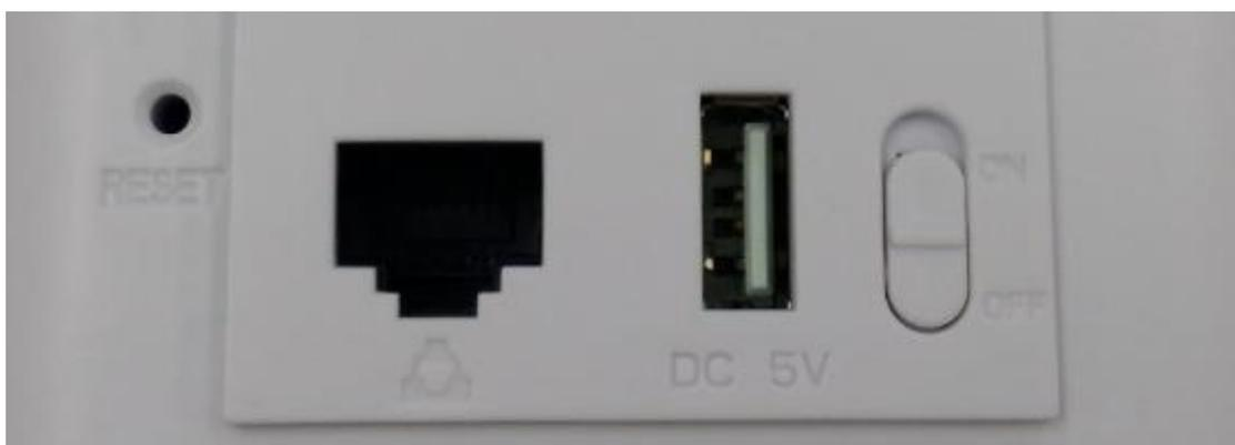
**Reset:** Press the Reset button about **15 seconds**, then release to reset
