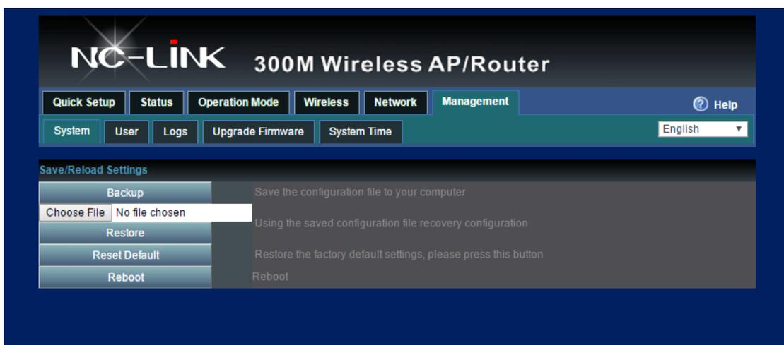
System: from here you can reload the backup file to restore the system, or restore to factory default, reboot the CPE through firmware
