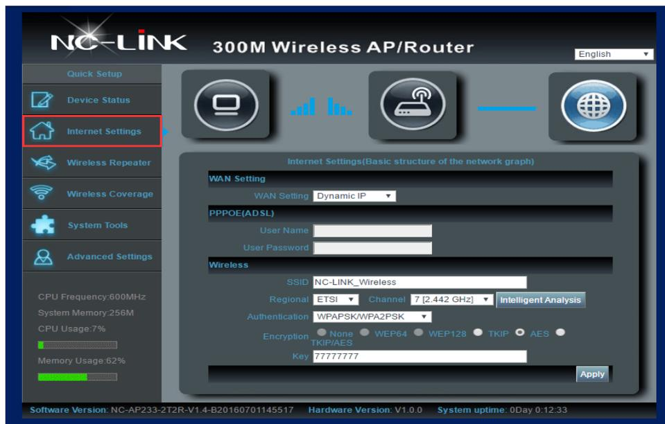
b) If Internet to LAN Port is **Dynamic IP**, only need to fill in the wireless parameters. Like **SSID, Authentication, Password**
